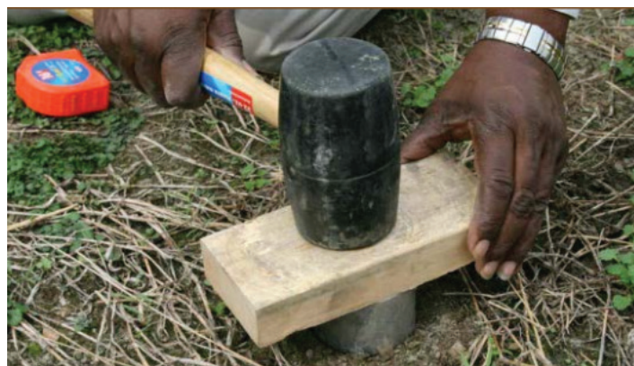
Sampling bulk density in the field with a soil core. Source: NRCS
