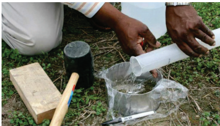
Water is poured into plastic-lined ring during an infiltration test. Source: NRCS
